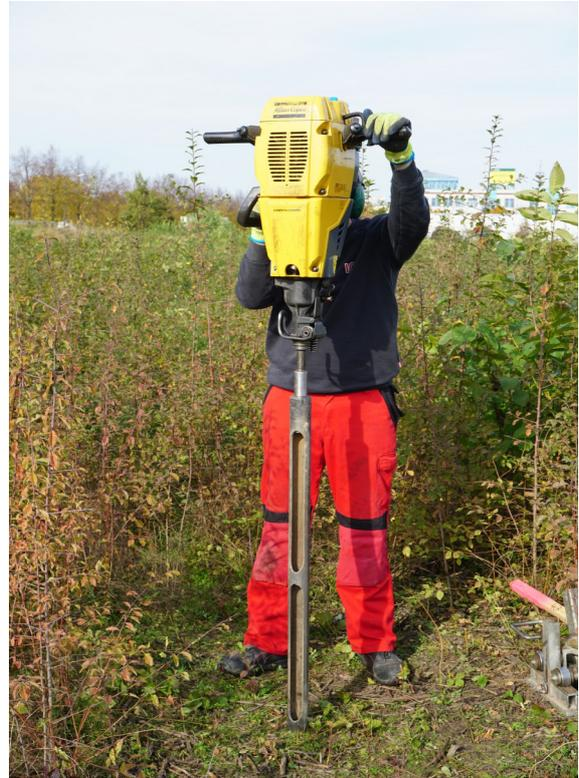
**Bild 2: A3 - Rammkernbohrung (RKB)**
